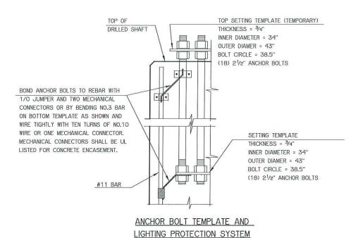
MONOTUBE STRUCTURE (DRILLED SHAFT DETAILS) (SHEET 3 OF 3) Detail JG JW
